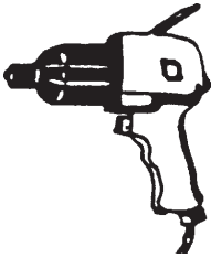
Fig. 8.11 : Hammer screw with pneumatic drive
