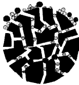
Fig. 5.13 : Adsorption material after 6 - 8 hrs drying time
