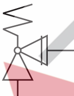
Fig. 9.6 : Diagram symbol for a safety valve
