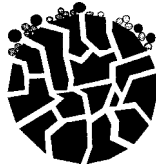
Fig. 5.11 : Adsorption material after 5 min. drying time
