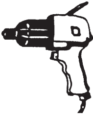
Fig. 7.4 : Drive screw powered by compressed air
